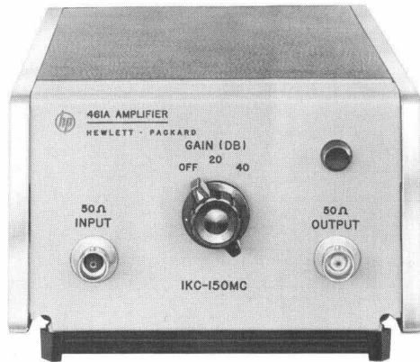
Fig. 3. Model 461A amplifier provides either 40 db (100 X) or 20 db (10 X) of broadband gain. Input and output impedances are both 50 ohms.
